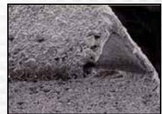
Diamond Delamination (Note: Large Grain Size)
