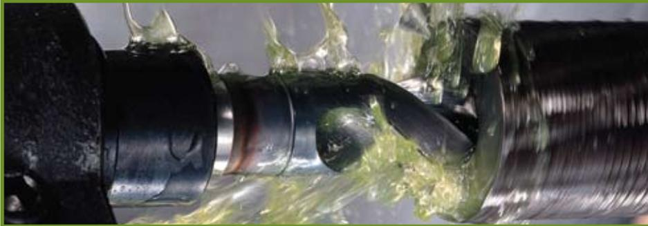
As our industry advances in technology, more options have become available on CNC machines for reducing cycle time. Decreases in machine time often generate profit. Elements that help decrease cycle time can range from high speed spindles and coolant-through capability to high-pressure coolant and Minimum Quantity Lubricant (MQL). With all of these options, one might ask, which is best for the shop?
