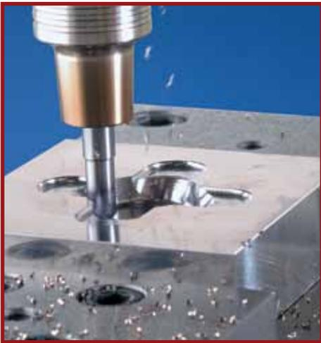
completed the whole rib milling operation with the end mill still in good shape. He checked all the dimensions and found everything to be per print. Then Jason looked at the timer and realized the operation completed in 9 hours and 42 minutes! He was very impressed with the run time, the finish, and the lack of significant wear on the end mill.
